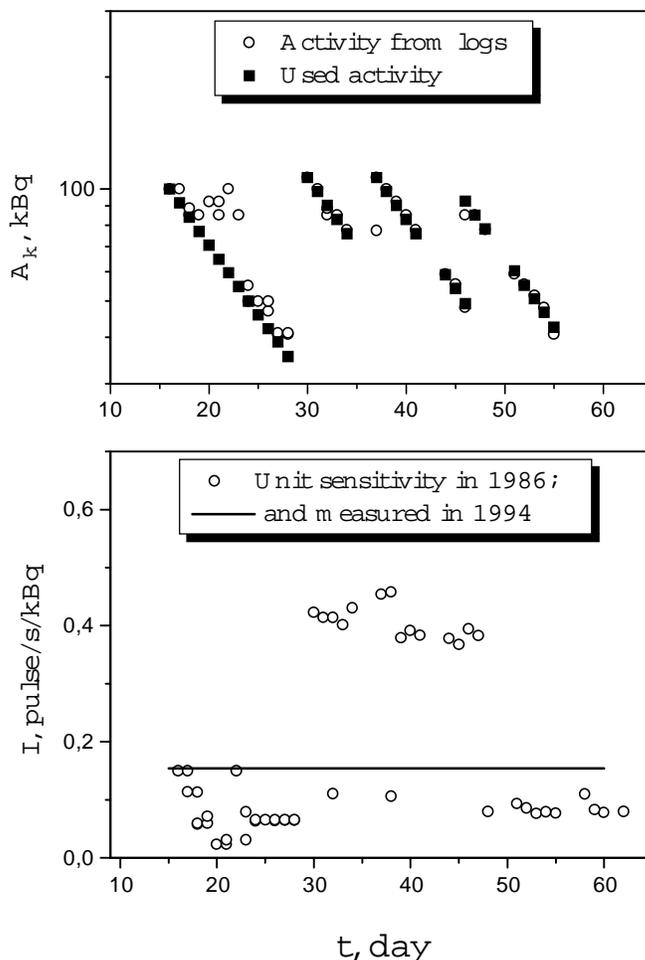
**Fig. 5.** Measurement of characteristics of the radiometric unit "Gamma" in 1986 estimated from records in logs and from our calibration data of 1994.  $A_k$  is the activity of  $^{131}\text{I}$  calibration source;  $I$  is the sensitivity of "Gamma" unit;  $t$  is the time after the accident.
