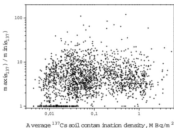
Fig. 2. Dependence of maximum measured  $^{137}\text{Cs}$  contamination density maximum ( $\sigma_{137}$ ) to the minimum ( $\sigma_{137}$ ) on average  $^{137}\text{Cs}$  soil contamination density.
