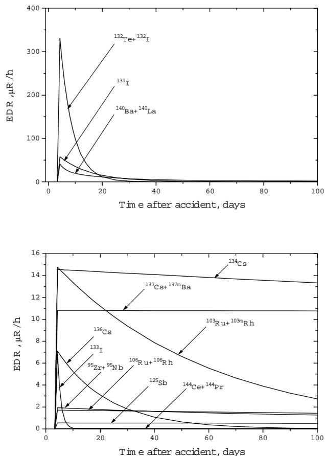
Fig. 1. Characteristic dependence of EDR at the height of 1 m from the ground surface for different radionuclides deposited in the Bryansk region (the <sup>137</sup>Cs contamination density is 37 kBq/m<sup>2</sup>).
