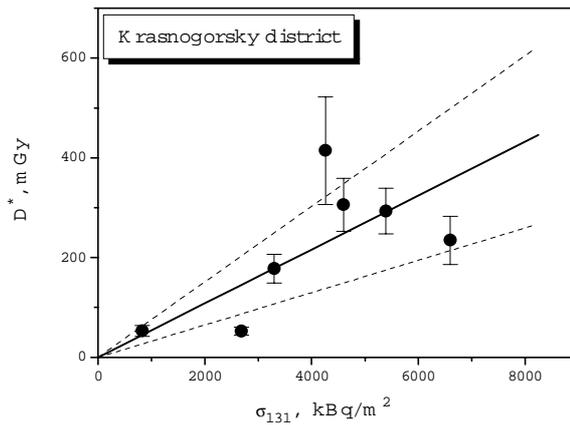
Fig. 6. Villages in Krasnogorsky area of the Bryansk region in which individual thyroid measurements were made (more than 9 persons). The statistical dependence between the average reduced thyroid dose and average  $^{131}\text{I}$  soil contamination density in a settlement. The dotted lines are 95% confidence bounds of the regression line.
