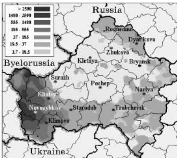
Fig. 4. Map of  $^{131}\text{I}$  ( $\text{kBq}/\text{m}^2$ ) contamination of the Bryansk region generated by the reconstructed average density. The contamination density is referred to 20 May 1986.
